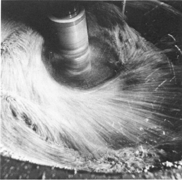
Fig. 3. Material streams in the intensive mixer.
